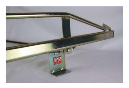
Again, these are very straightforward- they bolt into the ends of the cross bars with an M8 x 16 bolt with a spring washer.
