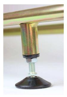
With there only being roof mountings at the front and middle of your van, the aft-most crossbar uses a pair of adjustable rubber feet instead and has an extra M6 Nyloc nut and bolt at the end to prevent it from turning. Drop this into place but again, don't tighten everything fully yet.
